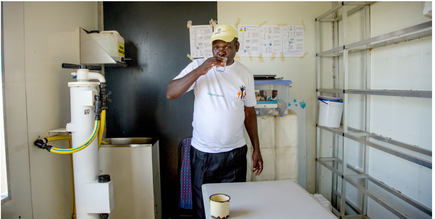
Inside a Safe Water Enterprise kiosk in Kenya with a SkyHydrant on the left.
